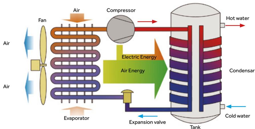
To understand the concept of heat pumps, imagine a refrigerator working in reverse. While a refrigerator removes heat from an enclosed box and expels that heat to the surrounding air, a HPWH takes the heat from surrounding air and transfers it to water in an enclosed tank.
